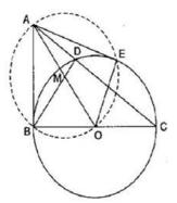
To construct : A right triangle ABC with AB = 6 cm, BC = 8 cm and  $\angle B = 90^\circ$  .BD is the perpendicular from B on AC and the tangents from A to this circle.
